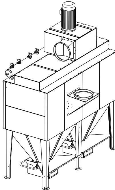
**Example of possible installation of FMC200-8L with QF duct connection and cellulose cartridges:**
