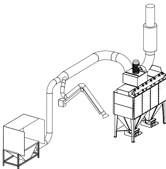
**Installation for extraction of welding fume and metallic dust.**
