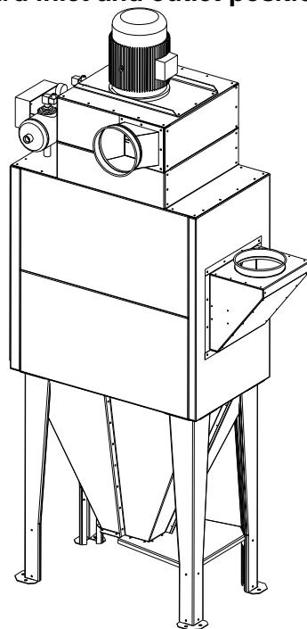
**Example of possible installation of FMC200-2L with QF duct connection and cellulose cartridges:**
