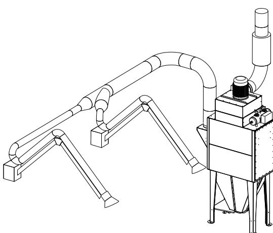
**Installation for extraction of welding fume.**
