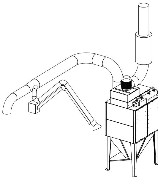
**Installation for extraction of welding fume and metallic dust.**
