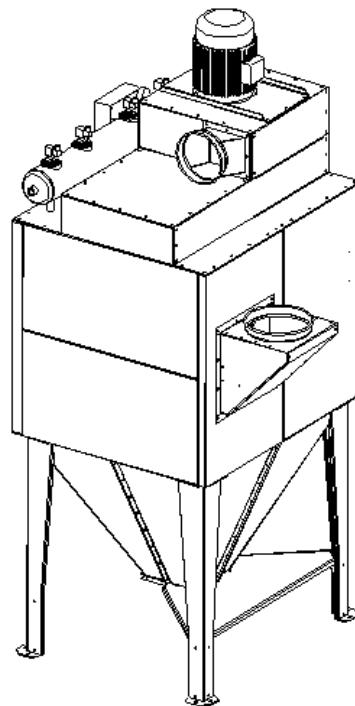
**Example of possible installation of FMC200-4L with QF duct connection and cellulose cartridges:**
