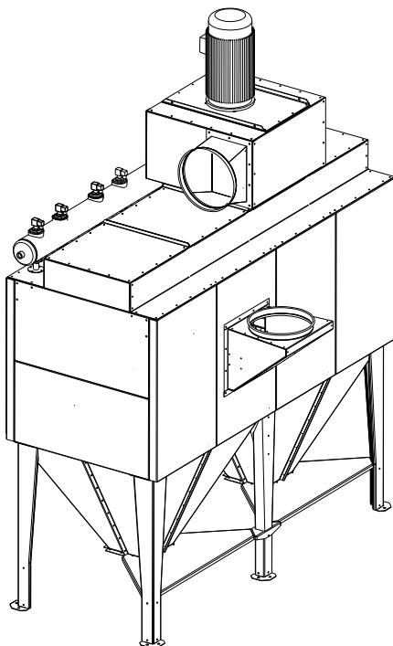
**Example of possible installation of FMK25-8L with QF duct connection and cellulose cartridges:**
