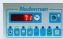
To simplify operation and maintain optimal performance, FilterMax is equipped with an automatic control system that operates and monitors the compressed air Pulse Jet cleaning process. The cleaning system is designed for maximum performance with minimum noise level. Different alarms notify if errors occur. The control system can also handle fans, dampers and dust feeding equipment.
