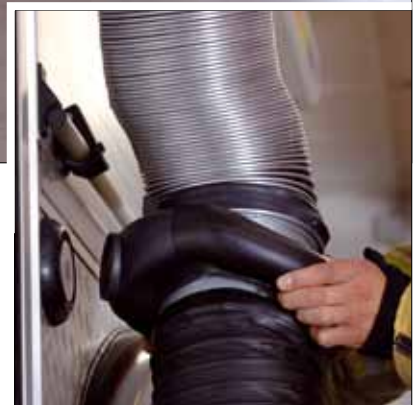
When activated, the electromagnet on the hose attaches to an anchor plate on the vehicle.
