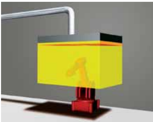
Fig.5 Robotic welding with canopy - low vacuum.
