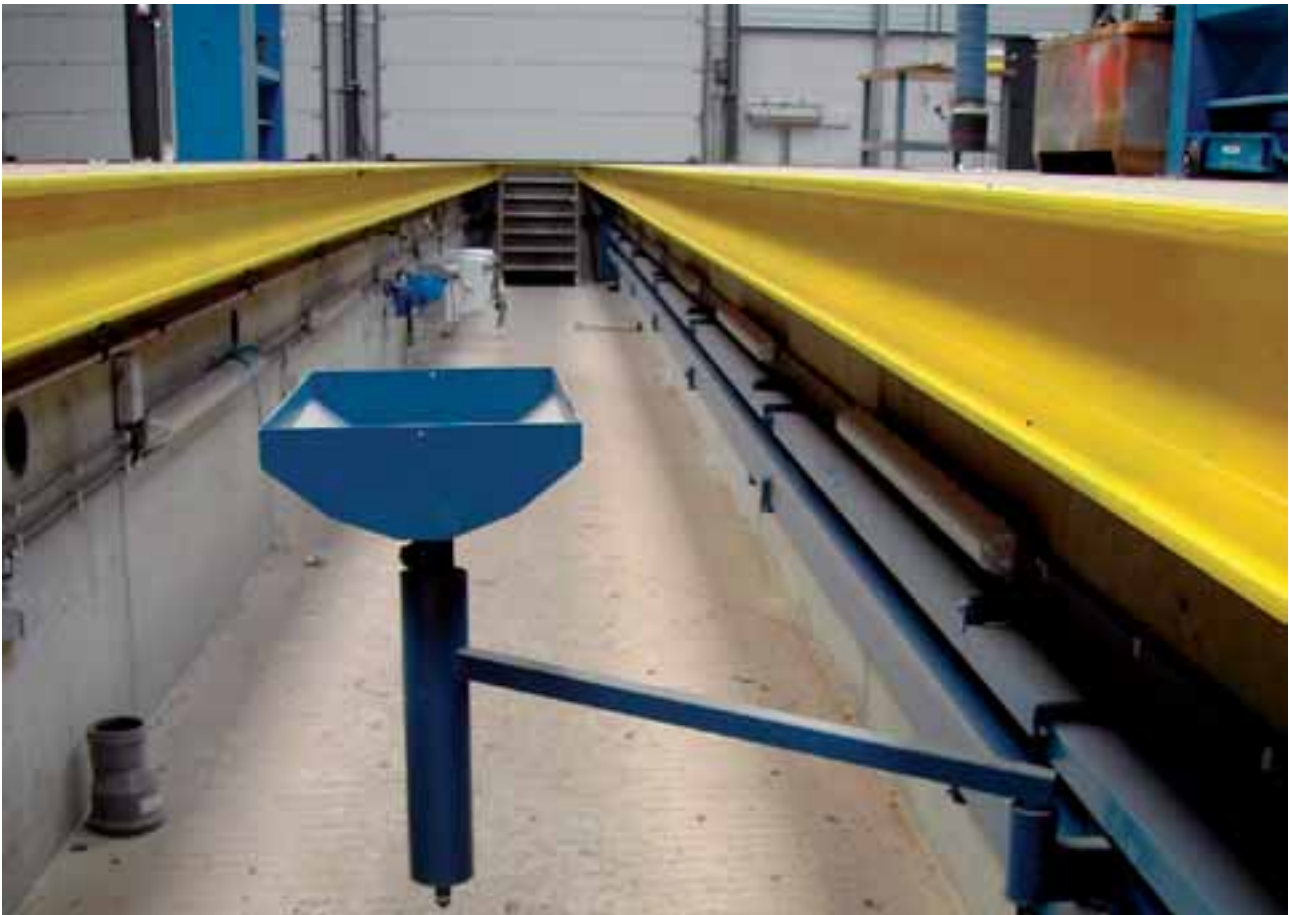
Fig. 4. Oil pitt fitted with Nederman fixed waste oil system. Hose reels for air, fluid and power.
