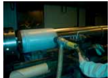
Fig. 4. On-tool vacuum blaster mounted on a lathe.
