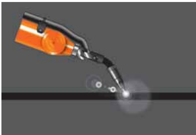
Fig.6 Robotic welding - high vacuum "on-torch".
