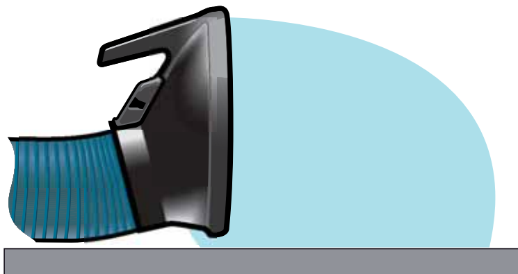
Fig.3 Using a flange and surface improves the suction field.
