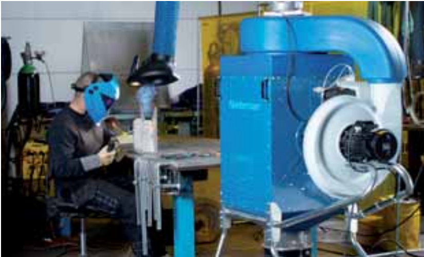
Fig 1. Proper positioning of extraction arm.
